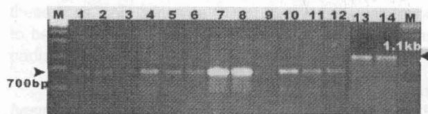
Figs. 3. (1-12: Amplification product of Lr24 marker; 13-14: amplification product of Lr9 marker) M: Marker lane: 1-6: Advanced lines of the cross HP1633/HP1776 (white seed), 7-8: Catalogued lines of Lr24 (red seed), 9-12: Catalogued lines of Lr24 (white seed) 13-14: Advanced lines of the cross HP1633/HP1776
