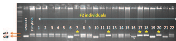
Fig. 1. Marker segregation of o16 -linked SSR, umc1149 among F 2 individuals of CML533 × QCL3024. Star marked individuals possess favourable o16 allele in homozygous state
